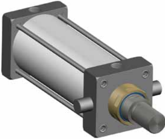
4" bore, 2" rod diameter, triple oversize Rod, with a one pcs steel head trunnion with cushion. ST3O3T1X-4X8-#2
