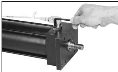
Bolt sensor to cylinder.
