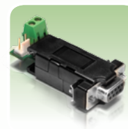
RS232-RS485 Converter Card Compatibility: Serial Port Used with: SP17C, SP23C, R256, R356, R525, BL100 RoHS Compliant Page 109
