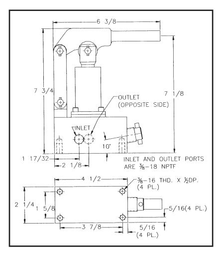
The series 500/50R modular hydraulic hand pumps are designed for use with an external hydraulic reservoir in a wide variety of demanding applications.
