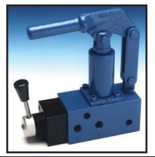
The hand pump with integral 4-way directional control valve incorporates a near zero leak shear seal manual type valve. The 4-way valve can control double acting cylinders or two separate cylinders from one pump. This style of pump can also include a reservoir and base plate to complete the hydraulic power package. There are several configurations for the 4-way including open center, closed center and tandem center. Contact our engineering department with your application specifics.
