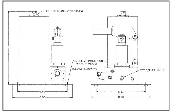
"L" = 7-3/4" for the 80 cubic inch reservoir and 13-1/2" for the 160 cubic inch size, consult the factory for custom size reservoir requirements.
