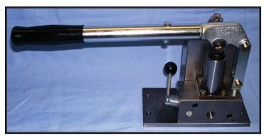
The package shown at the left is a modified pump and reservoir assembly. The customer needed a mount for mount interchange for an existing unit, so we provided a custom base plate, reservoir and also provided them with special plating on the linkage assembly. Our package reduced the number of strokes required for their application by 75%, improving overall efficiency.
