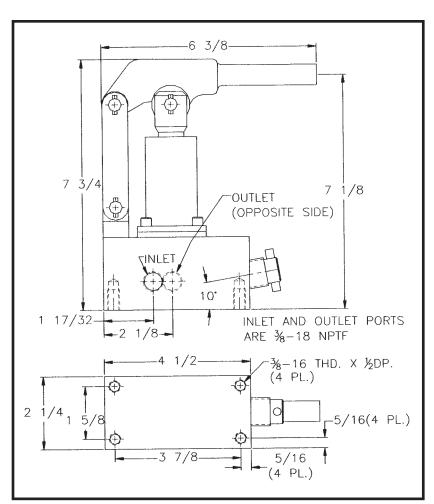
The series 550/55R two-stage modular hydraulic hand pumps are designed for use with an external hydraulic reservoir. The two-stage, or "HI-LOW", feature allows the operator to displace a larger amount of fluid at lower pressures. It automatically shifts over to a smaller displacement for higher pressures. This feature dramatically reduces cycle times, and number of strokes required, for many applications.
