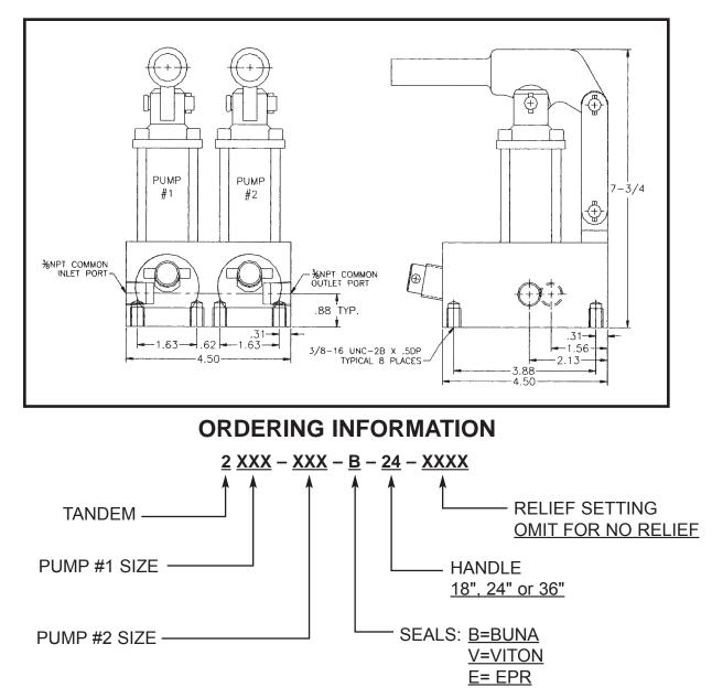
Standard sizes are 030 for 3/8, 040 for 1/2", 050 for 5/8", 060 for 3/4", 080 for 1", 120 for 1-1/2", 124 –125-126 are for two stage configurations. Any two size pumps can be combined, maximum pressure rating is a function of the final configuration, consult engineering for rating. When operated together the displacements and handle forces are cumulative, add for total displacement and force.
