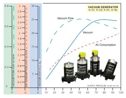
with a manifold subplate (sold separately) that mounts the complete module and provides #10-32 tapped holes for standard hose fittings. A single octoport gasket (included with the module), held in place by two mounting screws, insures a positive seal. Performance: Clippard modular vacuum generators provide high vacuum flow with high vacuum levels and are field adjustable. The adjustment screw at the base of the modular allows setting to the optimum performance needed to perform the task.
