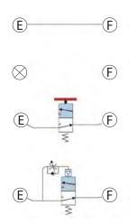
Maintained Output occurs as long as both palm buttons are held. Release of either button terminates the output (shipped in this configuration).
