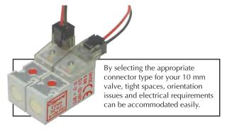
Another feature of the Clippard 10 mm valve is the ability to detach the coil and connector from the valve body. This can be useful for the purpose of orientating the coil by 180°, or exchanging connector types or voltages.
