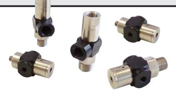
Pilot-Operated Check Valves work as standard check valves, but can be opened with an air pilot signal to permit free flow in the normally "checked" direction. The Clippard Pilot-Operated Check Valve provides the user with a reliable method to check flow in one direction, with the ability to remotely signal a free flow through the valve. Ideal for any circuit that requires this useful function-all in one valve that is easy to connect!
