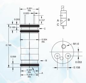
These direct actuating valves offer an extremely fast response time for accurate dosing of minute volumes with the same long life you expect from the original Clippard EV line of electronic valves, in a 8 mm cartridge package. Due to very low moving weights, they are extremely quiet and emit very little vibration. Subminiature size and low energy consumption make them ideal for many medical and diagnostic applications.
