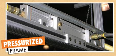
80/20 products allow you to customize workspaces to your people and processes. Design a station that can be adjusted up or down to accommodate the user; mount bins for storage or incorporate paneling to organize tools. What's more, you can create a pressure manifold in the T-slot channel so that a single hose can pressurize an entire frame, allowing you to add equipment where it's most convenient for you.
